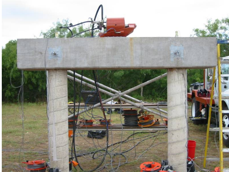
Figure 1.8 Shaker from Thumper was positioned at midspan of the beam
