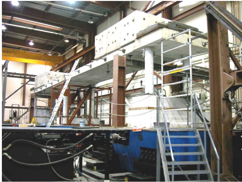
Figure 1.4 Shaking table specimen with deck and masses in place
