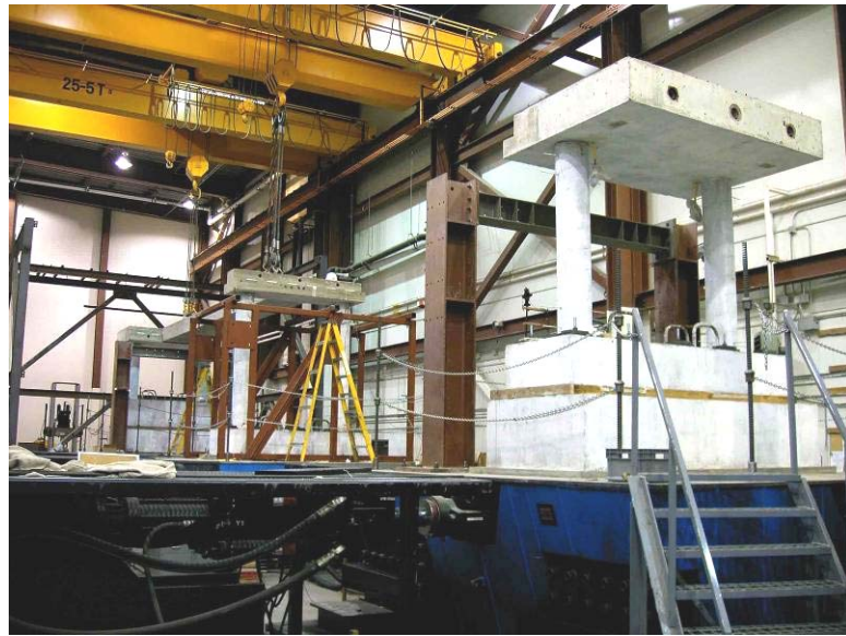
Figure 1.3 Bents positioned on the shaking tables at the University of Nevada, Reno
