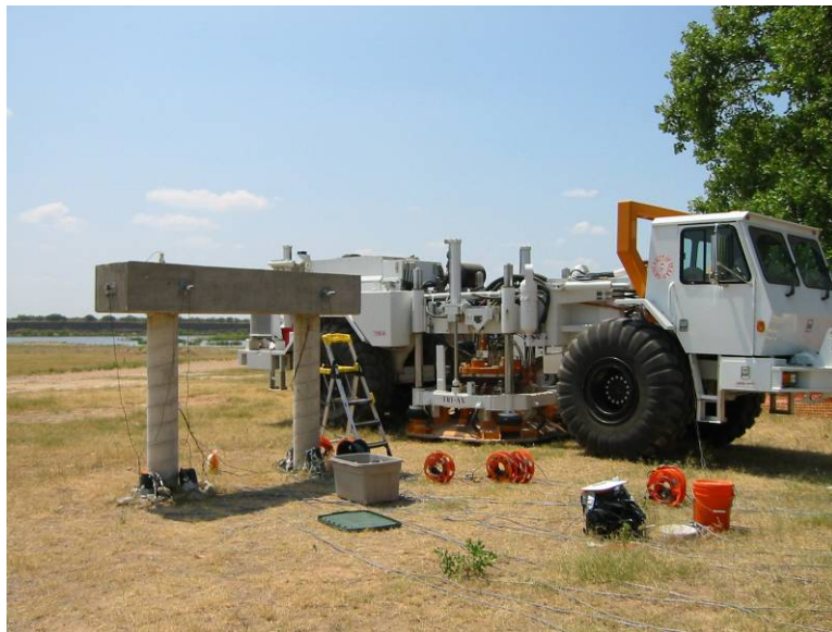
Figure 1.7 T-Rex was used to excite the ground surface in the vicinity of the field specimens
